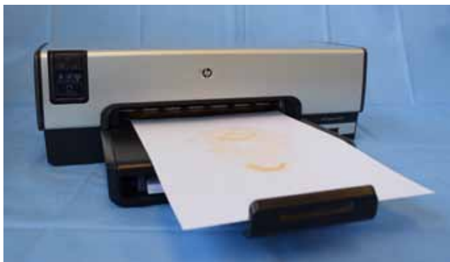
Figure 1: Standard HP Deskjet 6940 (Hewlett Packard, Palo Alto, Calif) office inkjet printer used for radiopaque printing with iodine enhanced ink.
