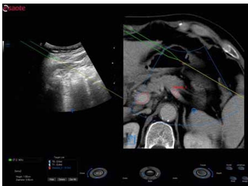
Figure 5 Real-time image fusion techniques allow ultrasound to be spatially co-registered with multiple volumetric image diagnostic modalities, such as those from MRI, CT, PET, and scintigraphy,
